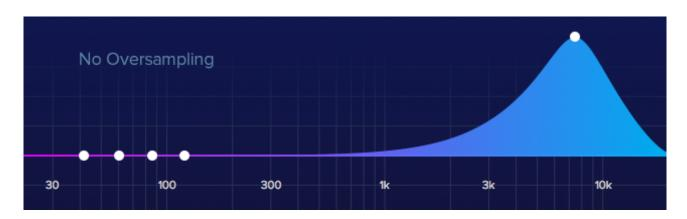
In this example you can see a peak filter set at 7.5KHz, 9dB of gain and 0.707 Q. Peak filters should be symmetrical but you can clearly see how it is not. On the right part of the filter you can see how the curve is distorted and it ends up at 0dB in the Nyquist frequency which is 22.05KHz.
