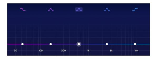
This is the main part of the interface. In this graphical display you see how each filter affects the incoming audio and you can also interact with it using the white dots in order to change the gain, frequency and Q.
